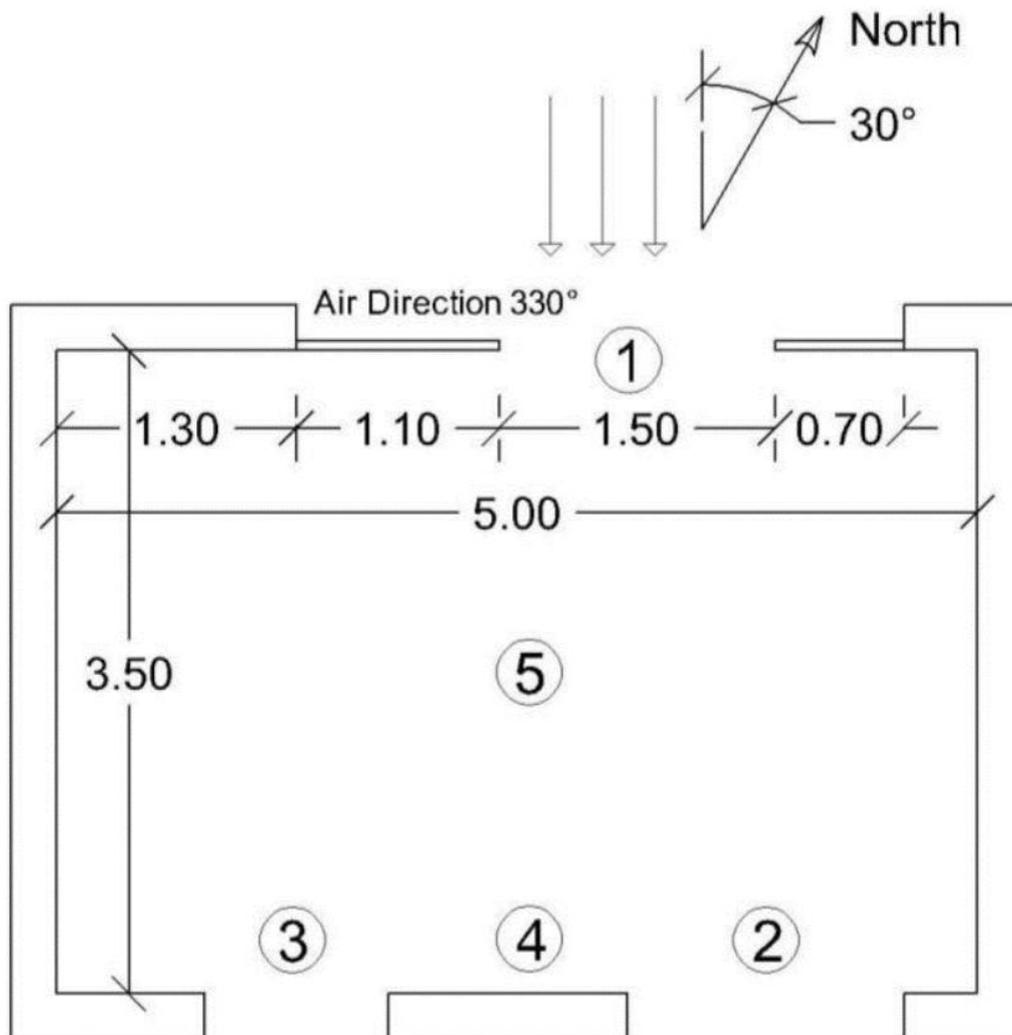
**Figure 9. Location of key points for indoor measurements.**
