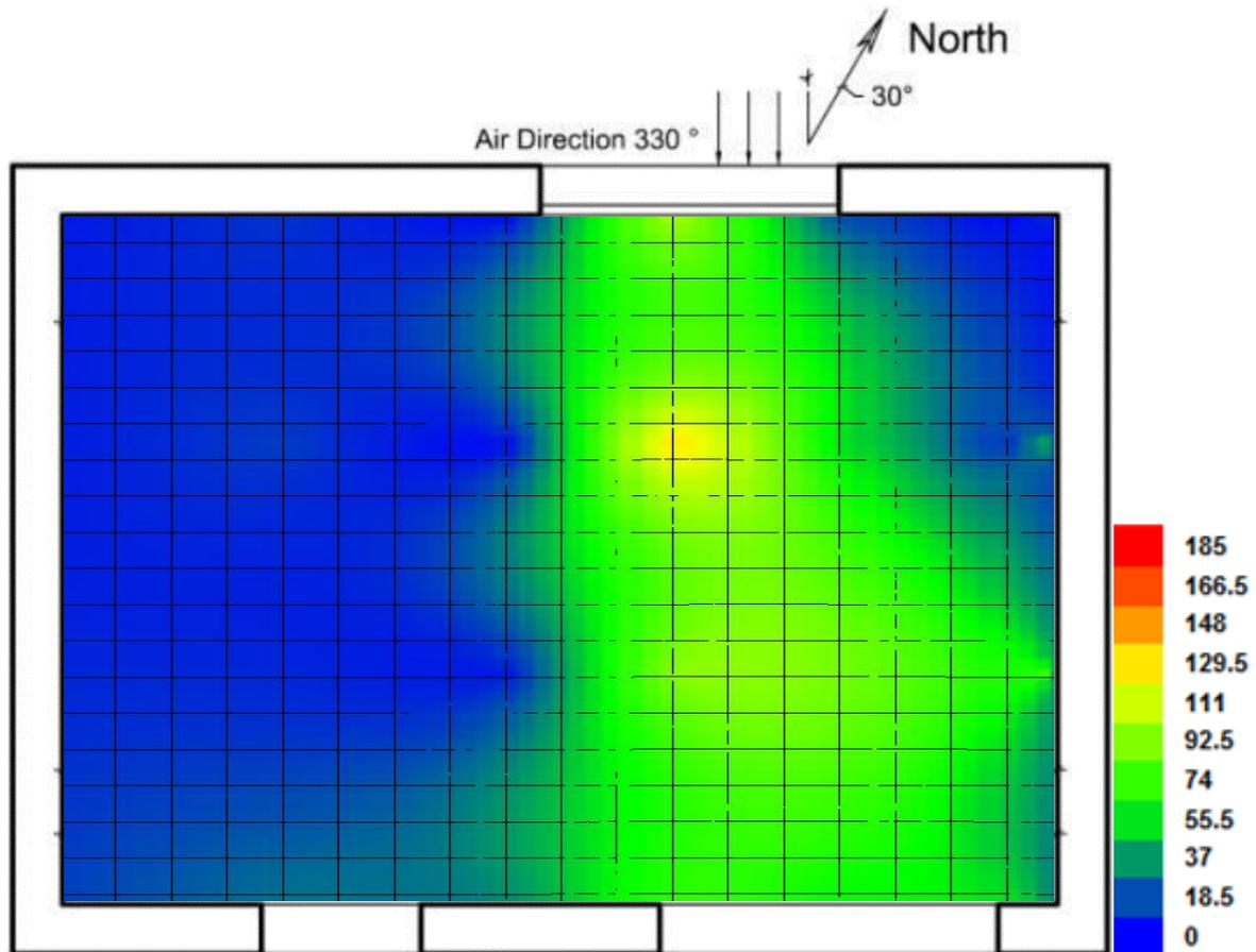
**Figure 12.**Contours for velocity magnitude as a percentage of wind speed, configuration C. Outside humidity (55%), temperature 25.5°C and wind speed of 5 m/s.
