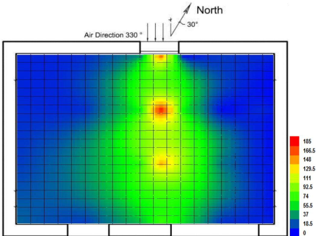
**Figure 11.**Contours for velocity magnitude as a percentage of wind speed, configuration B. Outside humidity (55%), temperature 25.5°C and wind speed of 5 m/s.
