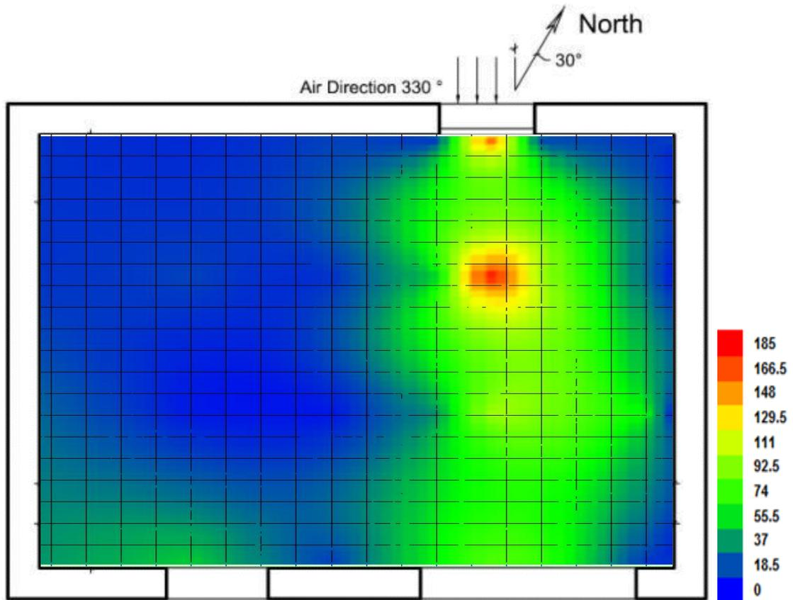
**Figure 10.**Contours for velocity magnitude as a percentage of wind speed, configuration A. Outside humidity (55%), temperature 25.5°C and wind speed of 5 m/s.
