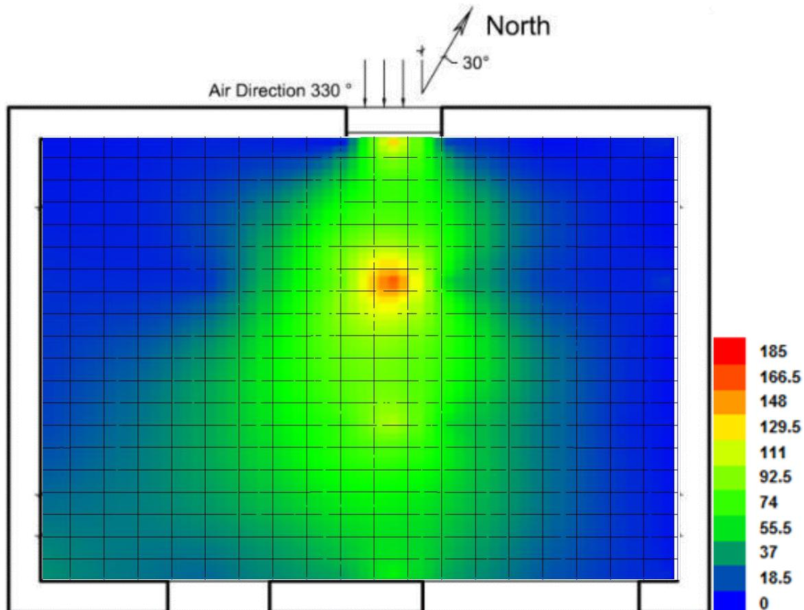
**Figure 13.**Contours for velocity magnitude as a percentage of wind speed, configuration B. Outside humidity (55%), temperature 25.5°C and wind speed of 3.5 m/s.
